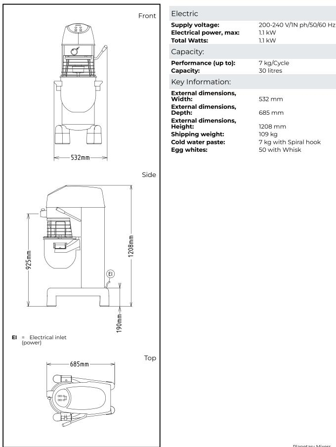
Planetary Mixers Planetary Mixer, 30 lt - Electronic with Hub
